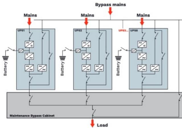
**CONFIGURATION PARALLELE ALLANT JUSQU'À 7 UNITES AVEC BYPASS CENTRALISE**
